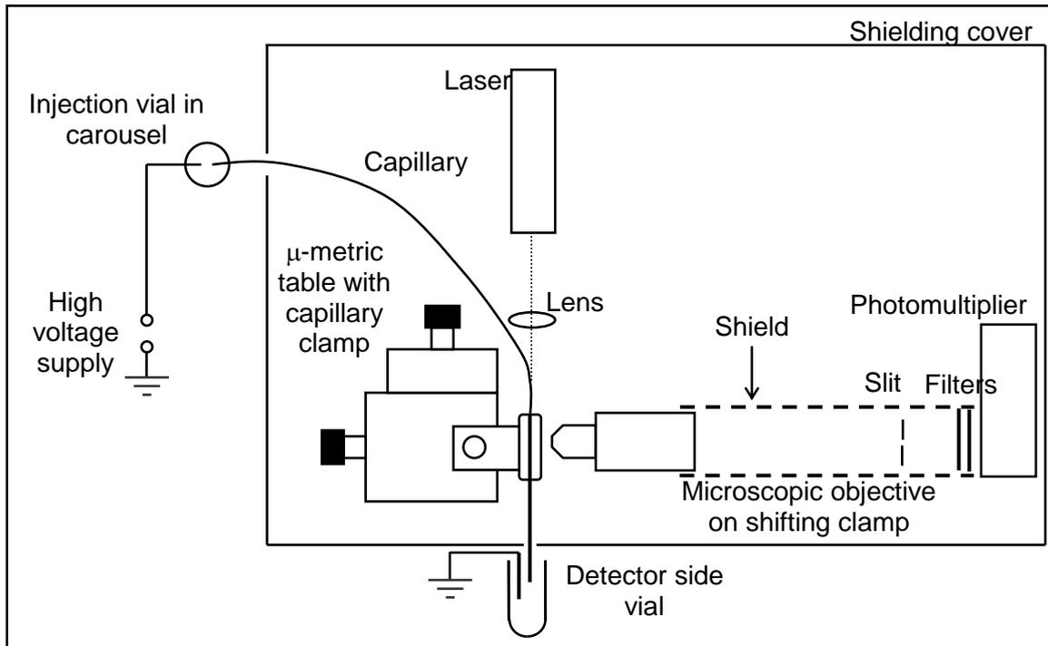
**Figure 3. Scheme of CELIF instrumentation.**
