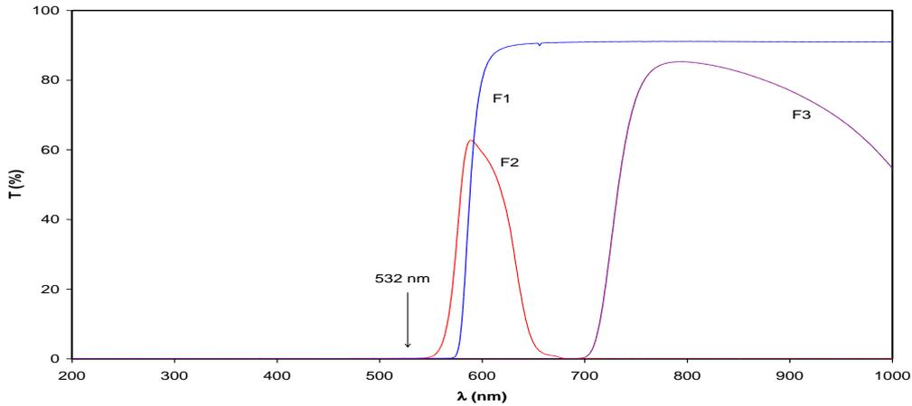
Figure 5a. Transmission spectra of selected optical filters
